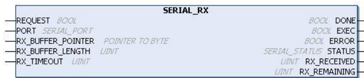
Figure 4-75. Block Used to Read the Reception Buffer Values
