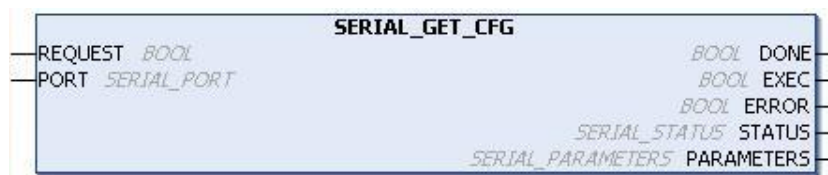
Figure 4-71. Block to Capture the Serial Configuration
