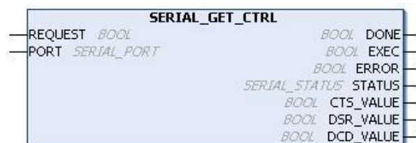
Figure 4-72. Block Used to Visualize the Control Signals
