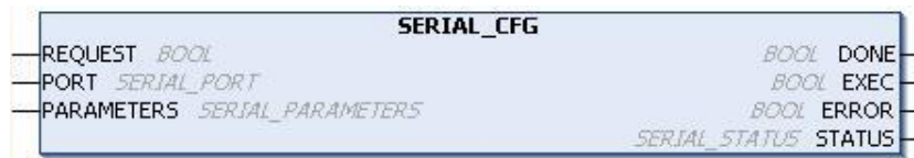
Figure 4-70. Serial Configuration Block
