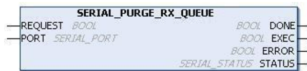
Figure 4-74. Block Used to Clean the RX Queue
