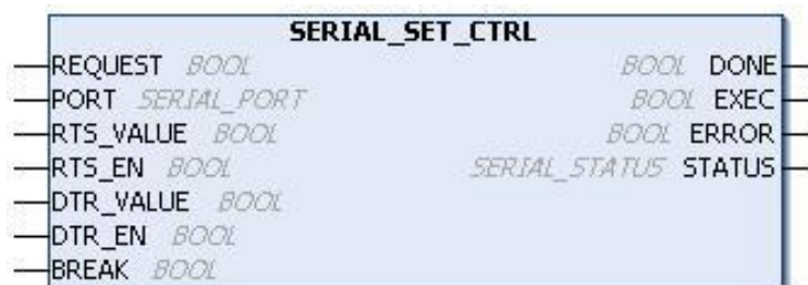
Figure 4-77. Block for Control Signals Writing
